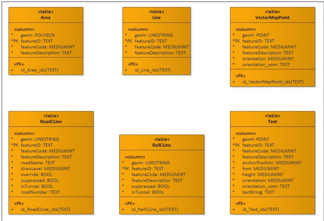
Figure 2: UML class diagram of the OS VectorMap Local feature types for the GeoPackage supply,
