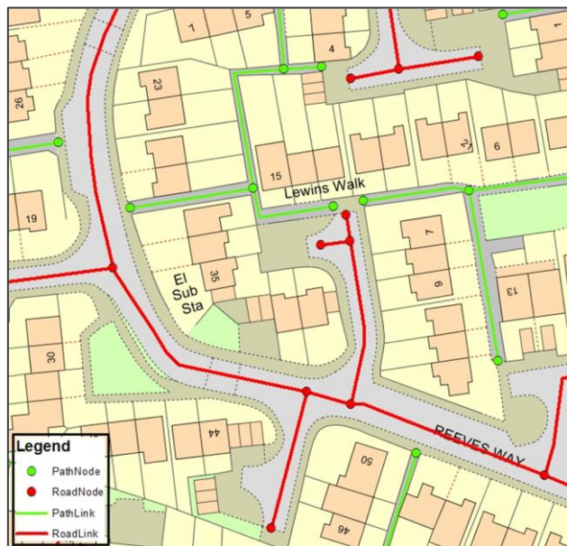
Figure 3: The road network and path network are not topologically structured together. They are independent networks.
