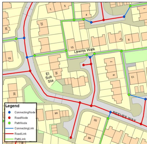
Figure 4: How Connecting Links and Connecting Nodes connect the road and path network together.
